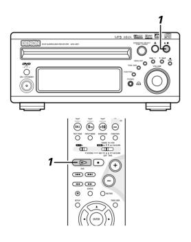
When the ADV-M51 is in the standby mode, the power can be turned on simply by pressing the play/pause button on the main unit or the DVD play button on the remote control unit. If a disc is loaded, playback starts.
